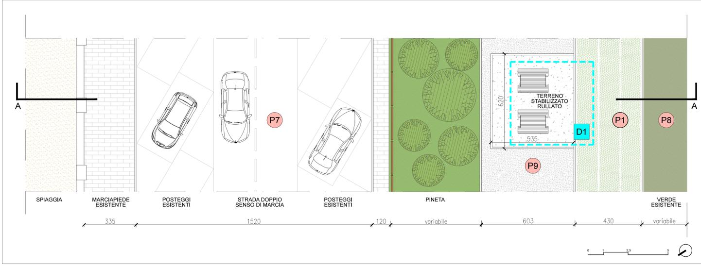
PINETA - PROGETTO: PIANTA TIPO AREA SOSTA ATTREZZATA - SCALA 1:100
