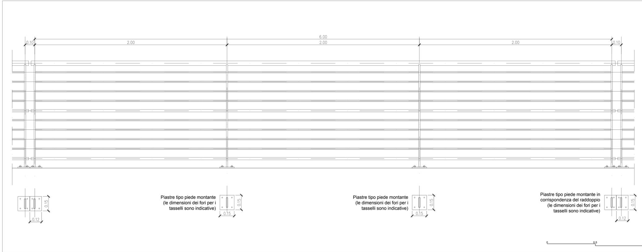
PROSPETTO TIPICO RINGHIERA IN CORTEN (FISSAGGIO SU CORDOLO) - MODULO DA MT. 6
